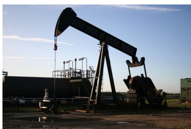
Figure 4: One of the oil pumps installed near the village for petroleum extraction. The machines are also known as nodding donkeys .
